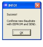
When the new baudrate information has been successfully sent, the sensor operates with the new baudrate. A window will pop up, prompting you to select **EEPROM** and then to press **SEND**. After a hardware reset the new baudrate only will be used when **EEPROM** and **SEND** have been pressed.
